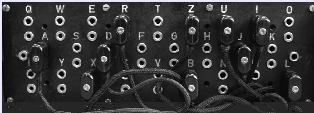
FIGURE 11-3 The Enigma steckerboard
